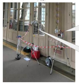
Microclimatic station for  $t_{db}$   $t_{wb}$   $v_a$  RH  $CO_2$  conc.
